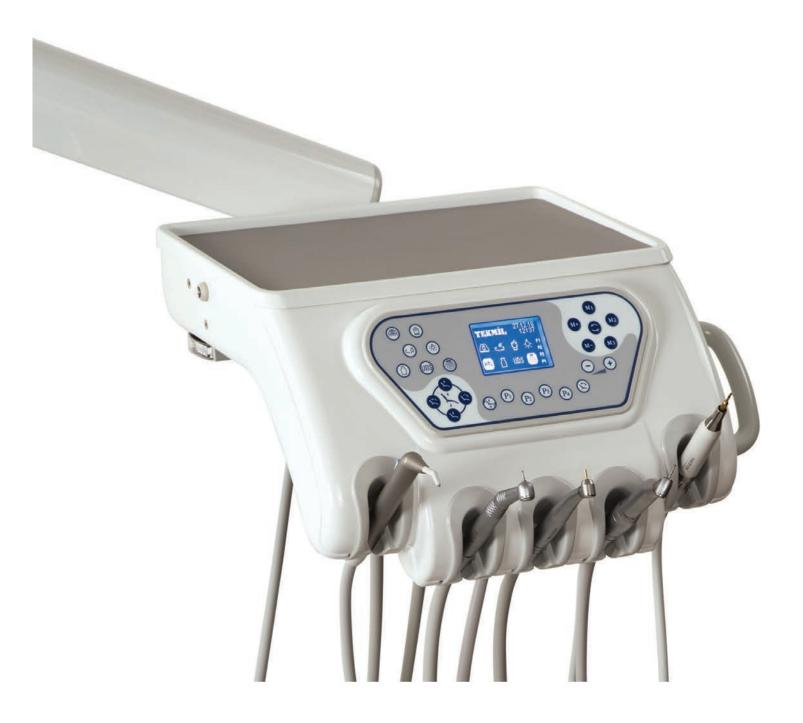
With an easy to use interface, with one button it is possible; cuspidor glass water on /off, selection of water tank or city water or unit disinfection system, working with water or without, peristaltic pump solution speed, chair movement control and chair movement programm.
